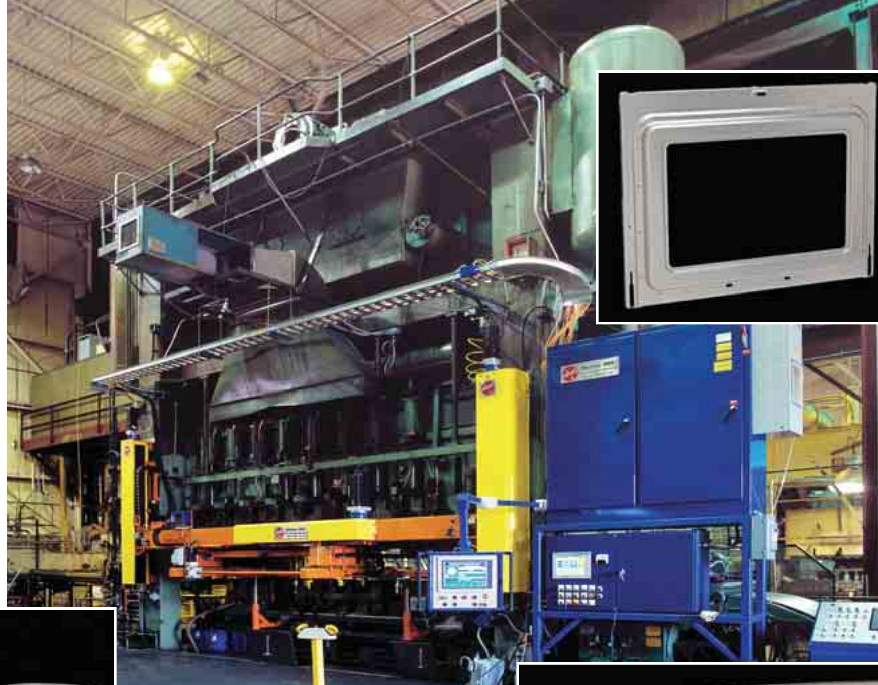
This 1200-ton mechanical press, outfitted with a new three-axis servo transfer system, produces more than 3 million parts per year—in various sizes, draw depths and material thicknesses—at the ICE Acklin Stamping plant. Parts include refrigeration compressor housings, shown at left with other Acklin stamped parts attached, and a stove inner panel and control panel (right).
