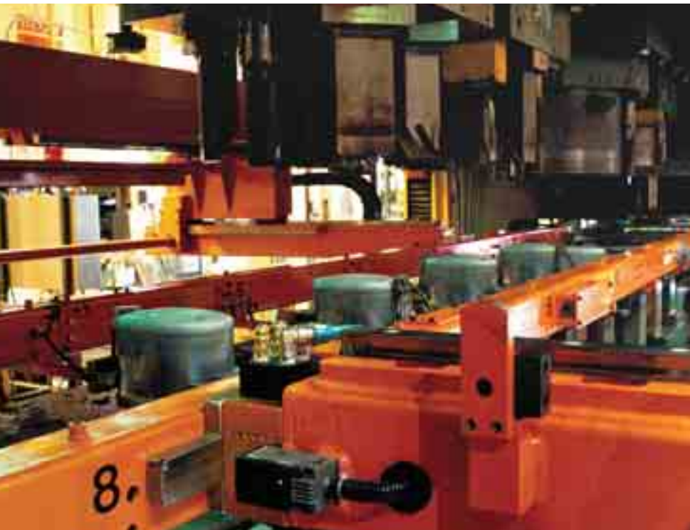
A new transfer system spans the 240-in.-long press bed and handles these thicker deep-drawn compressor housings as well as thinner, longer appliance parts. With the transfer came a new control package.
