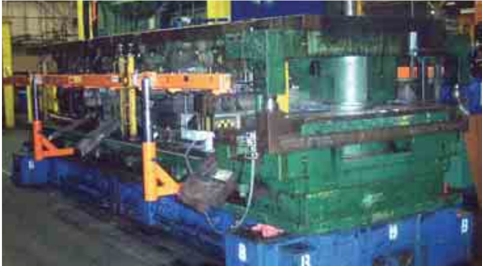
Transfer dies for the 1200-ton press are staged via one of two rolling bolsters, enabling 30 to 45-min. tool changeout between jobs.
